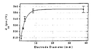
Figure 4: Effect of electrode diameter on the indirect d<sub>33</sub> of sample 1A
