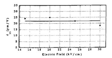
Figure 5: d<sub>33</sub> vs. Applied field for PVDF film
