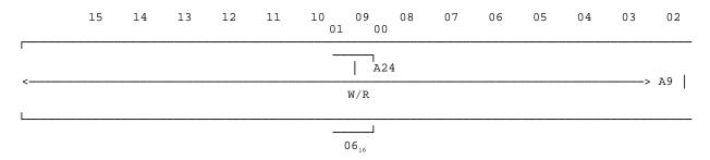
This 16-bit read/write register defines the base address of the A24 Operational Registers. The register is reset to an all "0" condition on power-up or the assertion of SYSRESET\*, and is written with the appropriate value under program control.
