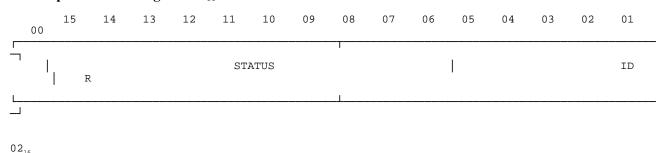
This is a read only 16-bit Interrupt Status Register. During an interrupt acknowledge cycle, this register will output a Status/ID value during a D8, D16, or a D32 data transfer. In a D32 data transfer, the upper 16-bits will be pulled up to logic A1@ by the backplane termination networks. A read from this register will show the current Status/ID value.
