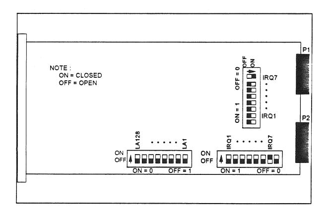
FIGURE 1 - V530 SWITCH AND STRAP LOCATIONS
