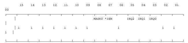
MASK0 (RW) ..... Interrupt Mask Bit for Interrupt Source
