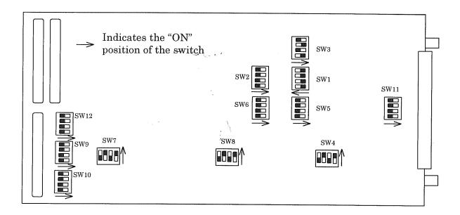
**Note:** For all the switch settings, a "1" representation for a setting indicates that the switch position is "Open" or "Off". A "0" representation for a setting indicates that the switch position is "Closed" or "On".
