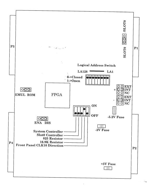
$\underline{Slot0\text{-}/Slot0\ Strap}$ : This strap is used to configure the adapter for Slot0 or non-Slot0 operations. Since the V157 does not support non-Slot0 operations, this strap must always be left in the  $\underline{Slot0}$  position.
