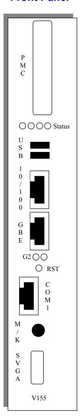
The V155 font-panel has all the standard external connections for monitor, mouse, keyboard, Ethernet, USB, and COM ports.
