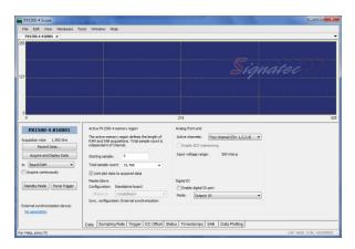
The PX1500 Scope App software is a virtual oscilloscope application that allows the operator to view or edit all digitizer hardware settings as well as record and display acquisition data.
