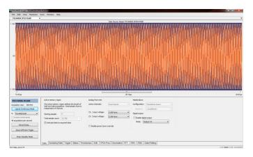
The PX14400 Scope App software is a virtual oscilloscope application that allows the operator to view or edit all digitizer hardware settings as well as record and display acquisition data.
