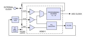
The synthesizer can generate any frequency from 45 to 128 MHz and most frequencies from 128 to 150 MHz. See the specification section for the range of un-settable frequencies.
