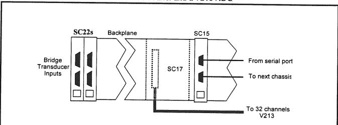
Note: The SC15-AB11 Serial Controller or the SC72-ZA11 Ethernet Controller with Calibrator and the SC17-AA21 Connector Adapter should be used with SC22 Bridge Signal Conditioners.
