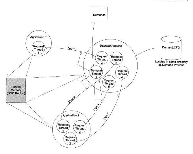
The demand process creates 1 named pipe with the name \\.\PIPE\DMDPROC. The multiple pipes shown in the drawing are multiple instances of the pipe \\.\PIPE\PMDPROC.
