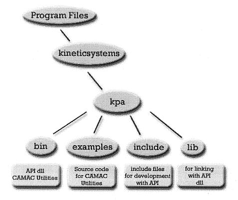
• <u>bin</u> This folder contains the API dll (kpaapi.dll), the Demand process (dmdproc.exe), the Demand statistics package (dmdsts.exe), an example demand configuration file (demand.cfg), and 3 simple CAMAC utilities (cam.exe, cactrl.exe, and costat.exe). The Demand and utilities software is described in different portions of this manual.
