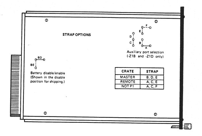
Before operation, move the strap from BD to BE (backup models). Note that the deep discharge protection circuit keeps the load disconnected until the plus six volts is applied, then removed. CAUTION: DO NOT GROUND THE STRAP WITH A TOOL. THIS WILL BLOW THE BATTERY FUSE.
