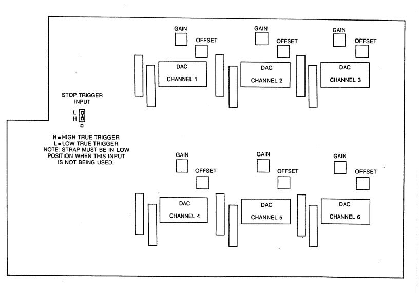
FIGURE 2 - OFFSET/GAIN CONTROLS
