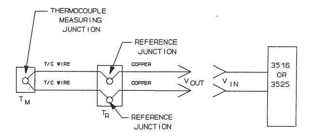
$T_{M}$  = Temperature being measured  $T_{R}$  = Temperature reference
