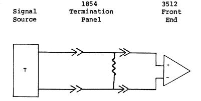
3. To connect current loop transmitters requiring a power source to Analog-to-Digital converter modules (active current loop operation). In this configuration, the power for the current loop is provided by the converter module:
