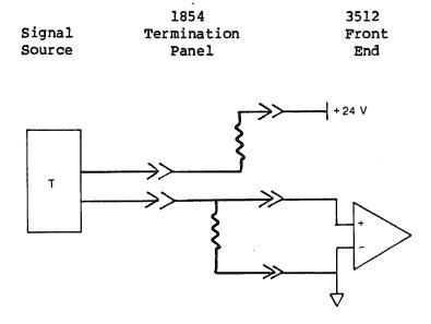
The Model 1854 is arranged so that each channel of the termination can be configured for any of the applications listed above. Thus, a mixture of differential voltage signals, and active and passive current loops can be attached to the same converter modules through the Model 1854.
