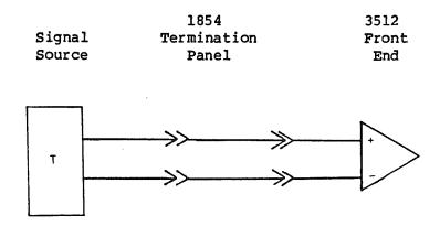
2. To connect powered current loop transmitters to Analog-to-Digital converter modules (passive current loop operation). In this configuration, the Model 1854 puts a 250 ohm precision resistor across the input signal lines to convert the current value to a measurable voltage:
