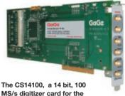
MS/s digitizer card for the PCI bus can monitor signals onboard an aircraft
