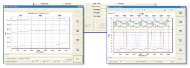
With a PLC and special software, the PV-1000 system measures, logs, and assists in binning wafers.
