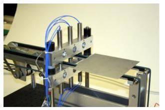
Three sets of push pull probes profile the PV wafer.
