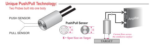
The Push-Pull probe is a unique version of MTI's Accumeasure™ amplifier series. This special design provides accurate surface information for wafer bow and warp.
