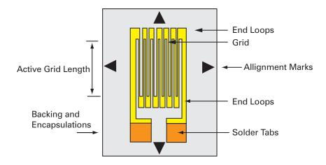
Small and low in cost, foil type strain gauges are the fundamental sensing element for many sensor types.
