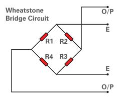
Assume E is the excitation supply input (DC) and O/P is the strain gauge's differential output. The O/P outputs pass to a strain gauge meter similar to a precision low-voltage DC voltmeter (Volts are calibrated to micro strain). The 1510A simulates this output voltage with up to 0.1 uV resolution. In this manner, users can check the stain gauge meter and adjust its span.
