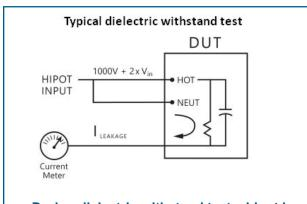
During dielectric-withstand tests, hipot is applied to both conductors and leakage is measured in return circuit through the ground connection.
