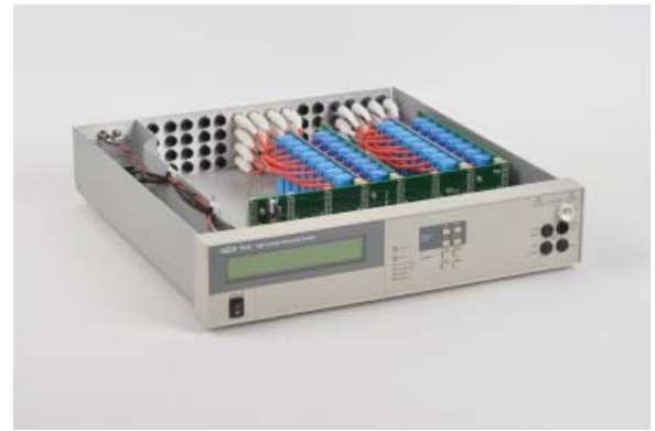
Figure 2. Vitrek 964i high-voltage scanning system
