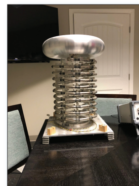
Figure 3 shows a 100:1 voltage divider network built in compliance with the NIST standard.
