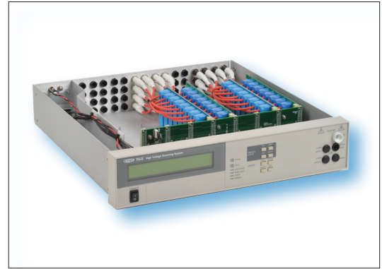
Figure 1. Open view of the Vitrek 964i highlights the unit's modular construction.
