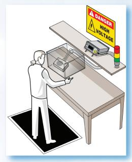
Figure 7a & b. Alternative setups for bench-top hipot test
