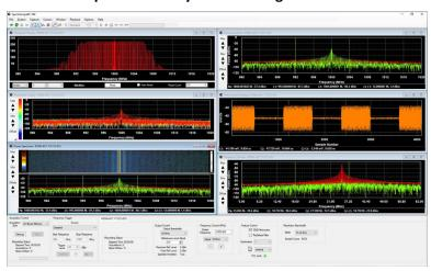
SpectraScopeRT, the Windows based spectrum analyzer application that requires no programming and allows for integrated operational control of both the downconverter receiver and the digitizer for signal capture, analysis, and real-time streaming signal recordings, has now been enhanced with the following new feature updates:
