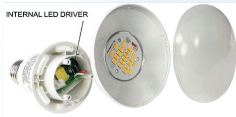
Figure 1. Input/output power of a driver integrated into a LED fixture must be monitored to measure against the IES LM-79-19 for efficiency.
