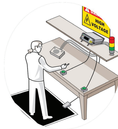
Figure 5. Example of a safe workstation set up for high-voltage testing.
