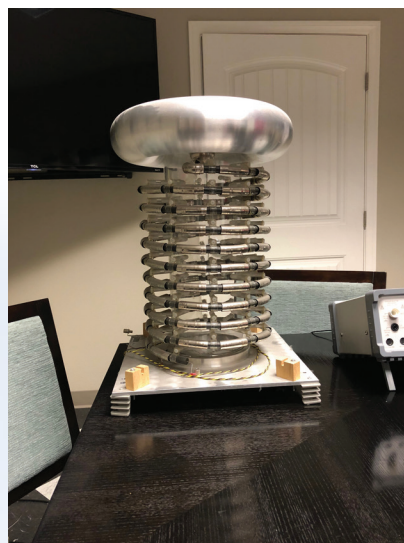
Figure 1. Example of a typical voltage divider network.
