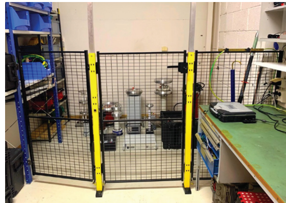
Figure 4. Example of a fenced-in work area for testing high-voltage equipment.
